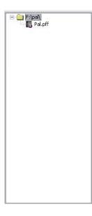
A database is identified by the red and gray AirSpeed Multi Stream icon. It also has a .pff file extension.
